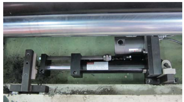
Electrical Actuator AD-24 is used on a Printing Machine for Unwinding
